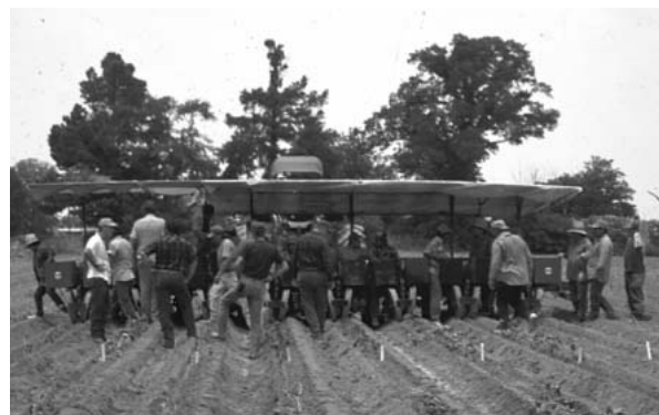
An eight-row sweetpotato planter at rest in Louisiana. A tractor pulls the planter manned with 16 laborers who insert cuttings into the machine for automatic planting. (Photo courtesy of Dr. Don LaBonte, Louisiana State University)
