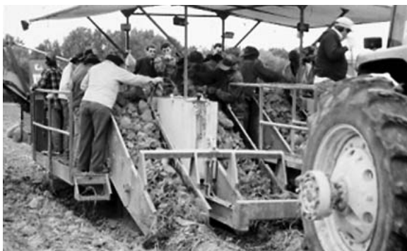
A four-row harvester at work in Louisiana using 23 workers to harvest 5 ha (12 ac) per day. Sweetpotatoes are graded, and put directly by conveyor belt into 360 kg (800 lb) crates for transport to curing sheds. (Photo courtesy of Dr. Don LaBonte, Louisiana State University)
